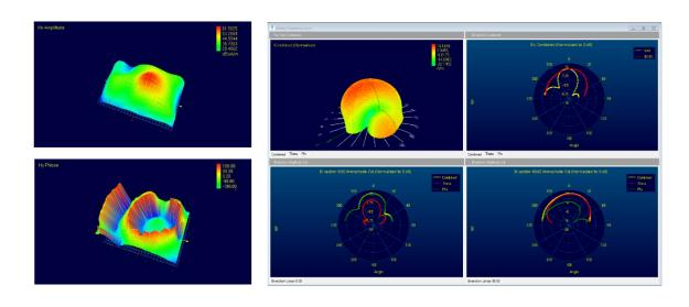
With the Circular Polarization (CP) option, the RFS calculates the right and left hand circularly polarized patterns and displays axial ratio patterns. RFS can be integrated into virtually any automated test bed and production line by using DLL programming.
